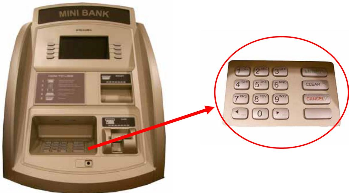
Fig 3.3 LCD & Customer Keypad
