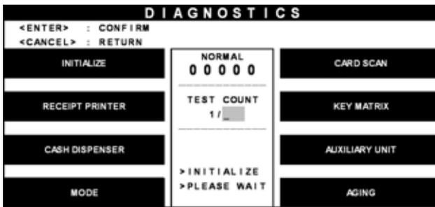
2) Select 'CARD SCAN' in the DIAGNOSTICS menu. And if the display is ready, please insert and remove the card quickly.
