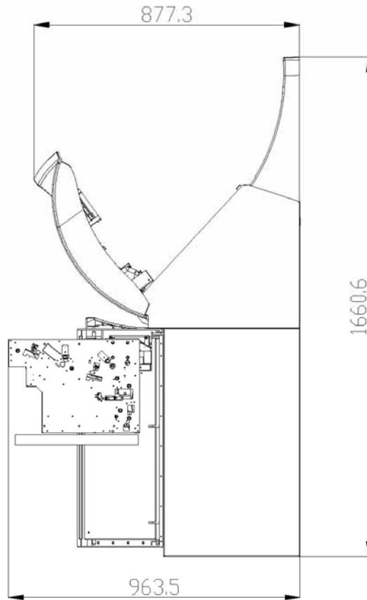
Fig. 4.2 Installation space #2 (Side view)
