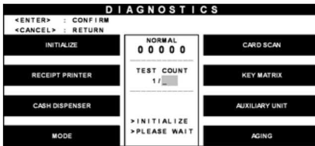
2) Select the 'RECEIPT PRINTER' in the DIAGNOSTICS menu. Test String will be printed from the receipt printer.
