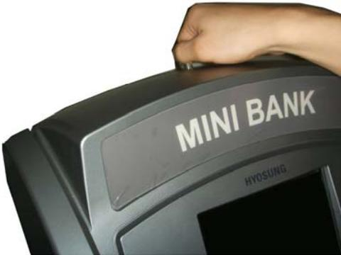
1) Insert the Front Panel key and turn it clockwise.
