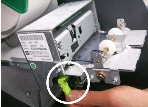
1) Open the Front Panel with key and pull this outward completely with hands. To remove a jammed paper inside transport path, press the green lever down to release the lower roller assembly.
