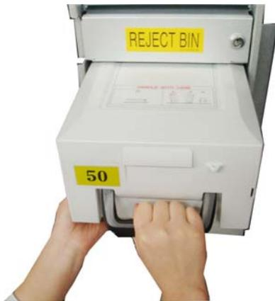
7) With one hand holding the cassette handle and the other hand supporting the cassette from the bottom, place the cassette carefully on the set guide of the CDU and push it in until it is locked in place.
