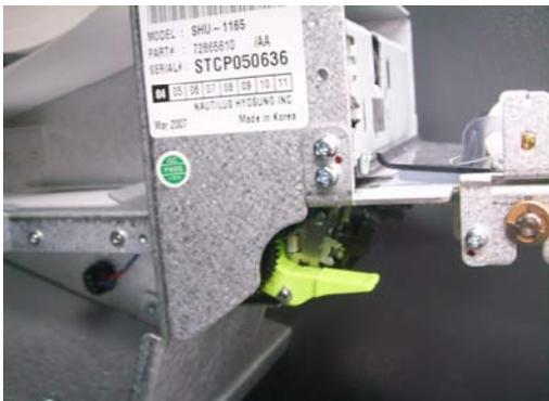
6) If the paper does not feed at all during initializing, make sure that paper has a CLEAN CUT at the end and the green lever behind the transport path is on its right place (It must not be lifted up).
