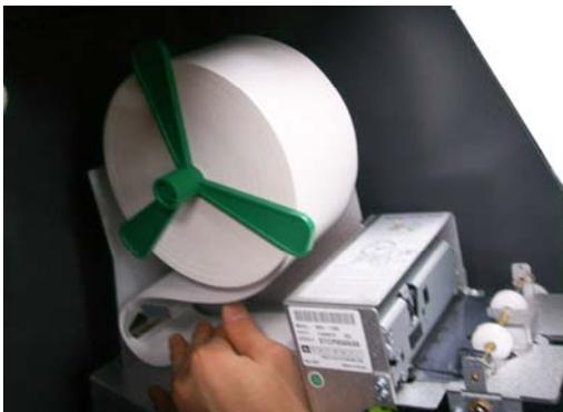
5) Insert the leading edge of paper into the loading guide of the receipt printer slowly. When the machine is initialized, the paper is going to start feeding
