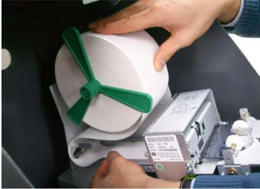
4) The shiny side of the paper should be faced up to be printed properly and the metallic tension guide should be surrounded with paper to reduce the tension during feeding
