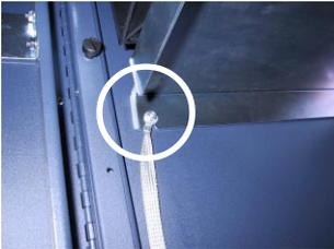
*Grounding strap secured to dispenser tray mounting bolt.*
