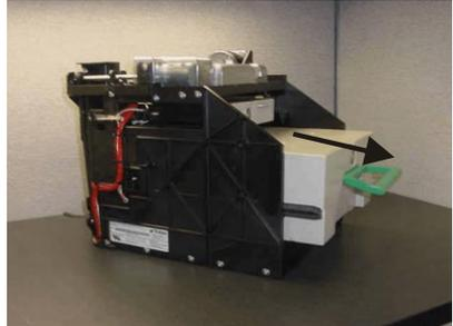
*Figure 4-6b. Removing note cassette. (TDM-150)*
