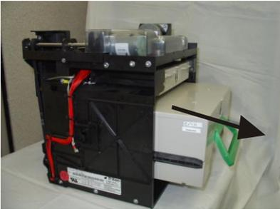
*Figure 4-6a. Removing note cassette. (TDM-100)*
